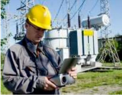
Detecting corona discharge has not been easy for utility engineers, until now. This article describes UV camera technology designed to detect the radiation emanating from corona discharge, how to inspect and view corona in daylight, and how to document and create a site report.
