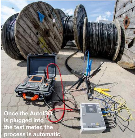
Once the AutoISO is plugged into the test meter, the process is automatic
