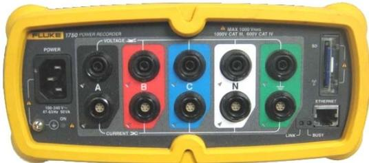
**Photo 3 - Three-phase voltage with common reference, ground connection provides capability for neutral-ground voltage, 5-current channels (3-phases plus neutral and ground). AC measurements only, no DC capability.**
