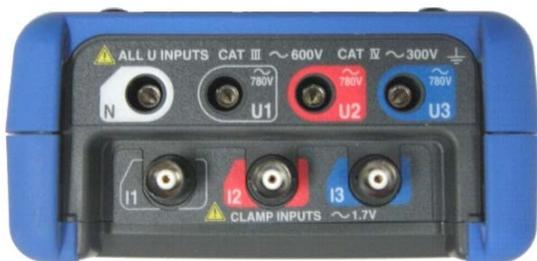
**Photo 1 - Three-phase voltage with common reference (phase-neutral), no neutral-ground voltage, 3-phase currents and calculated neutral current. AC measurements only, no DC capability.**
