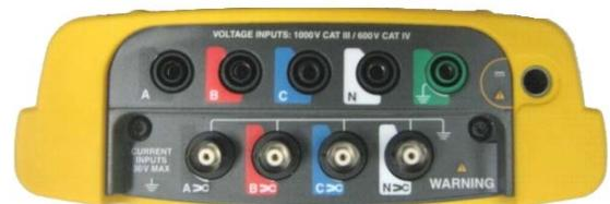
**Photo 2 - Three-phase voltage with common reference, ground connection provides capability for neutral-ground voltage, 4-current channels (3-phases plus neutral). AC measurements only, no DC capability.**
